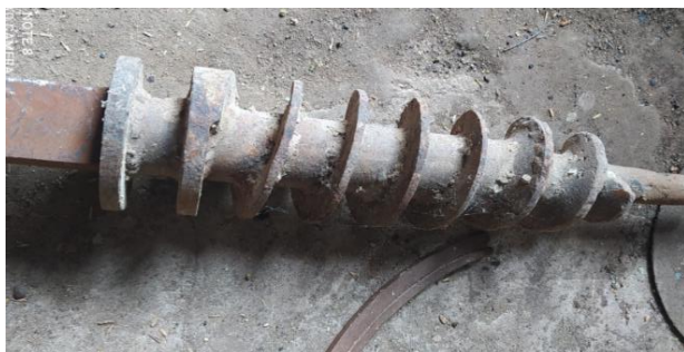
Figure 23 Screw of current briquette processing equipment
