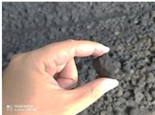
Figure 51 Particle size of delivered coal
