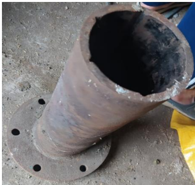
Figure 21 Nozzle of a briquette machine
