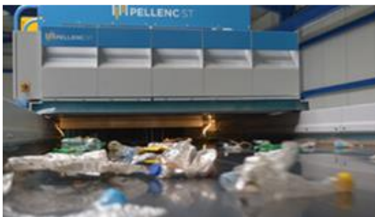
Figure 77 Identification by reflected light in the near-infrared
