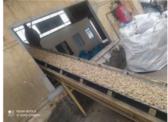
Figure 57 Slag Discharge System at the bottom of furnace (right), Conveyor to feed Rice Husk Pellet (left)
