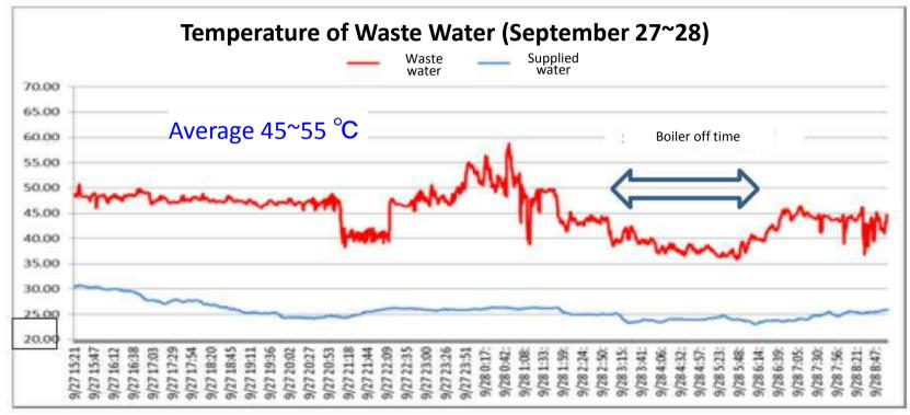
This is the temperature of all waste water from process machines and measured at the point outside of the workshop. The temperature of waste water at the dropping point of machines is far higher than the above temperature.
