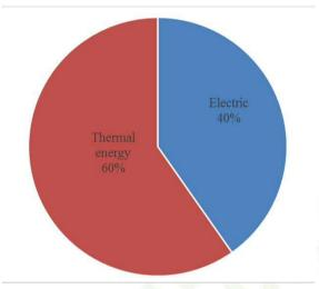
**Energy consumption structure in textile plant**
