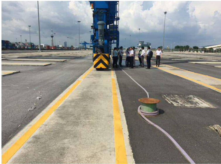
Photo 13: RTG cable deployed on road surface
