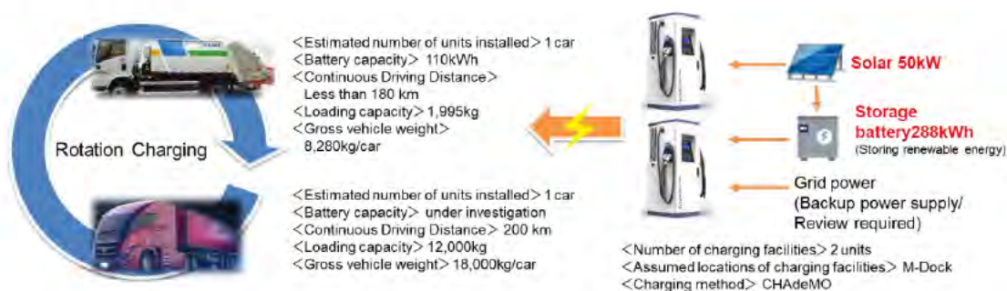
Figure 3-6 : EV waste transportation vehicle and charging system to be considered for introduction
