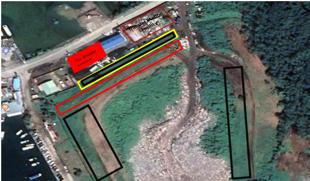
Figure 3-5 : Planned solar panel installation at a resource separation and Transshipment storage facility
