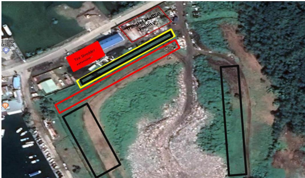
Figure 3-3 : Planned solar panel installation at a resource separation and Transshipment storage facility
