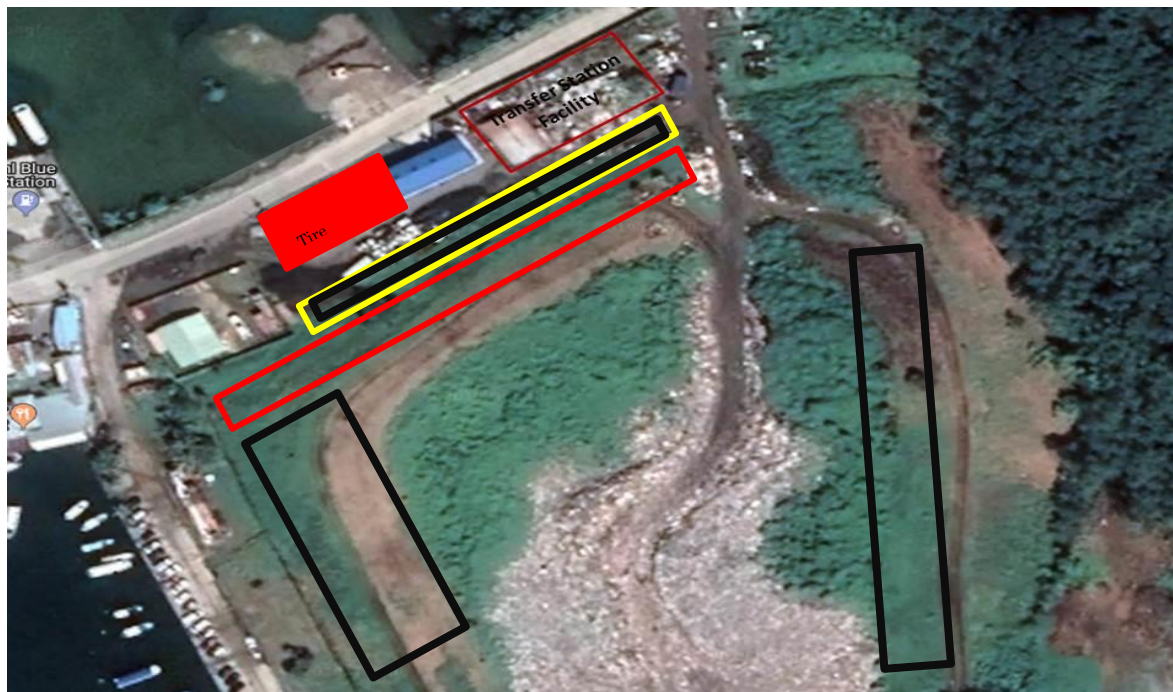
Figure 1. Bird's eye view of M-Dock Landfill site. Location for the planned Transportation Station Project. Red boxes indicate locations for installation of solar PV panels. Black boxes are potential areas to install additional solar PV panels. Yellow box indicates available roofed parking space (parking space can accommodate more than 20 large vehicles and a charging station) and additional rooftop space for PV panels.
