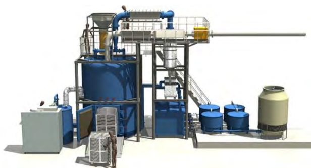
Figure4-3 : Urban Rig (UARBAN-RIG / URC-150, Processing capacity of 15 t/15m 3 per day)
