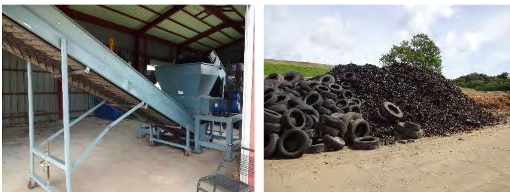
Figure4-1 : Scrap tire processing facility in Koror State at M-DOCK's former final disposal site(Left) Shredder and conveyor belt, (Right) Shredded tire chips
