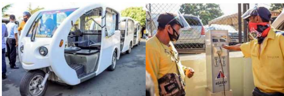
Figure 4-13 Charging Station for E-Trike
