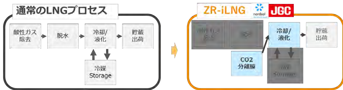
Figure 3-6 Comparison between existing LNG conversion technologies and ZR-iLNG technology
