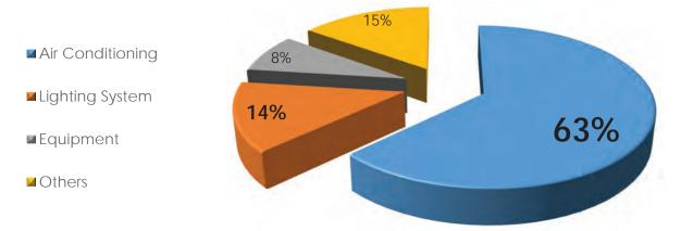
63% OF POWER CONSUMPTION BY KLCH BUILDINGS IS FROM AIR CONDITIONING SYSTEM
