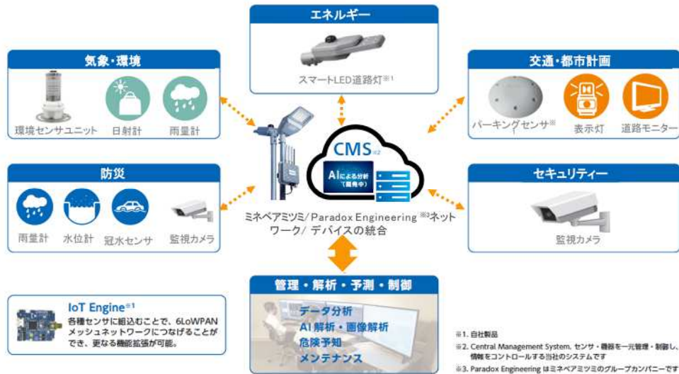
Figure 6-5 Examples of Functions that can be Added to Make Smart Streetlights
