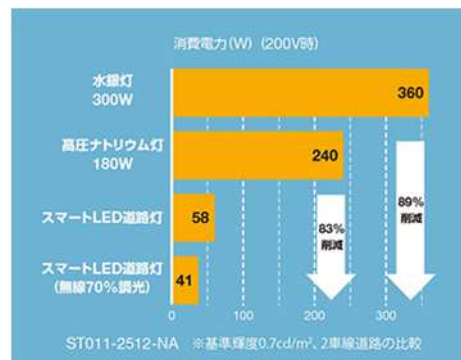
Figure 6-4 Energy Saving Impacts of High-Efficiency LED Streetlights
