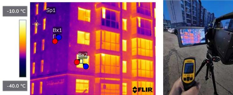
Figure 4-17 Confirmation of Heat Loss by Thermographic Measurement
