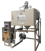
Photo 3.2.4.3 BDF production system (batch type)
