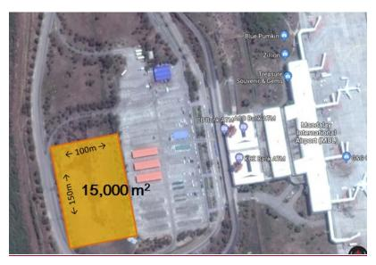
Figure.2-7. Assumed installation location of solar panel for estimation.
