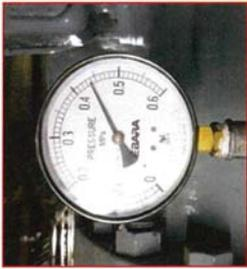
Discharge pressure gauge = 0.44 MPa
