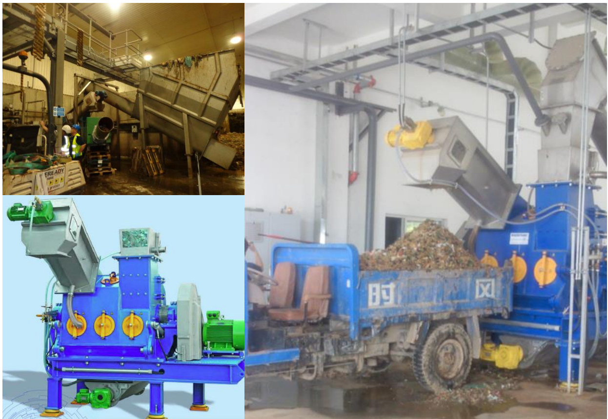
Fig. 2-6-15: Example of Fracturing/ Filtering with Hammer Mill
