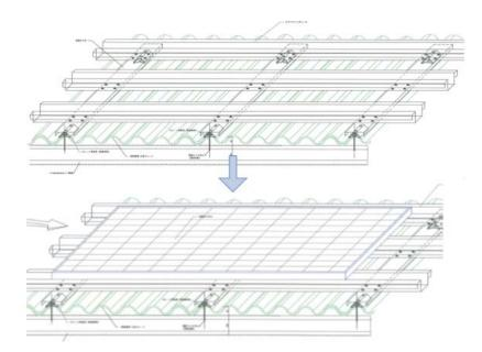
Figure 3.2.2-10 Ultra light installation method (slate roof) (Source: Prepared from Kawaguchi Steel Industrial Mounting Procedure Diagram)
