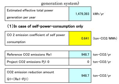
(Source: Created from application form for Public Interest Foundation Corporation Global Environment Centre Foundation) [Calculation of CO2 reduction effect by introducing high efficiency chiller]
