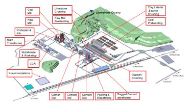
Figure 3.4.2-1 General layout of cement factory (Source: From the presentation materials of Chip Mong Insee Cement)
