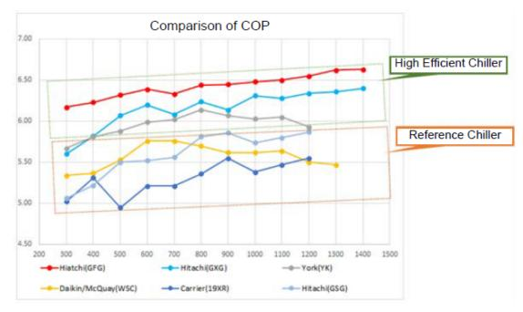
Figure 3.3. 2-5 COP comparison of Hitachi GFG and reference equipment
