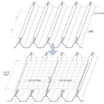
Exhibit 3.2.2-9 Ultra light installation method (folded-plate roof)
