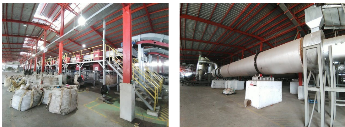
Figure 2.3.1.3.6. Sorting line (left) and rotary kiln dryer (right) at Kesiman Kertalangu TPST RDF production facility (Source: Photos by survey team)
