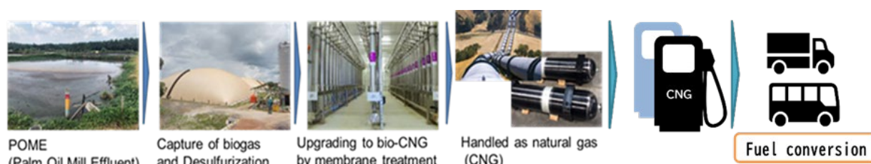
Figure 4-3 Overall image of project for POME biogas utilization
