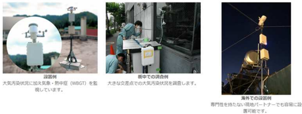
Figure 5-16 Examples of air quality monitoring using fixed-point sensors
