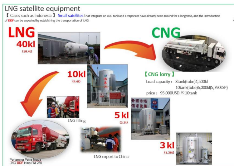
Figure 4-7 LNG satellite equipment lineup and CNG supply
