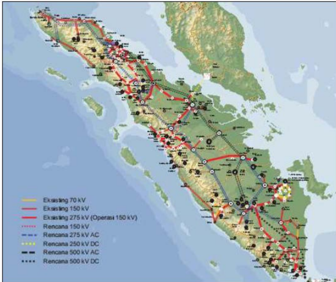
Figure 9 Sumatra island power transmission network development plan 4
