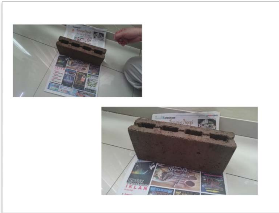
Figure3-14: Blocks for building materials made from residue (prototype)
