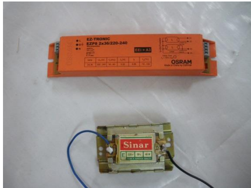
Photo 6: Copper-iron ballast (below) and electronic ballast (above)
