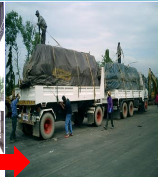
Cover solid waste and transfer to sanitary landfill (60 trucks)
