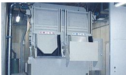
Figure 2-6 Volume reduction and solidification facility for temporary storage of organic waste
