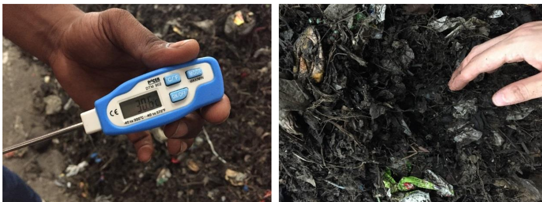
Figure 3-11: Compost Heap Temperature (Left ) and Final Compost Product (Right) (Taken at a BBMP Facility. The temperature is not high enough and final compost is immature)
