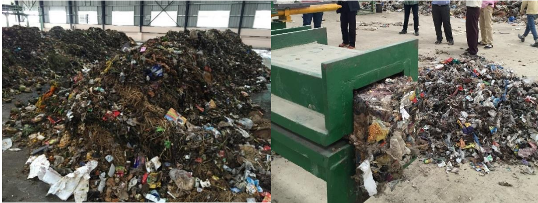
Figure 3-18: Composting Organic Waste (left), bailing residue of plastic (right)
