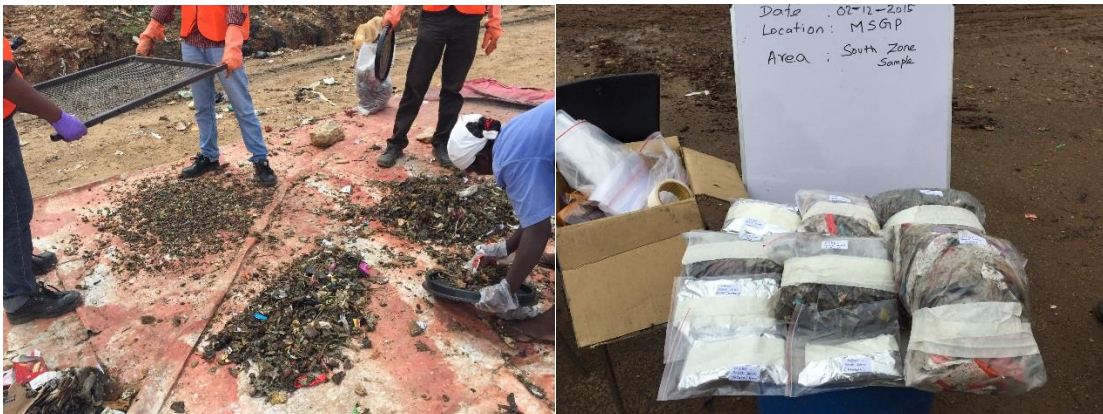
Figure 3-4: Categorization of “Woods and Grasses” and “Soil and Sand” (right) and packaged samples for the further analysis (left)
