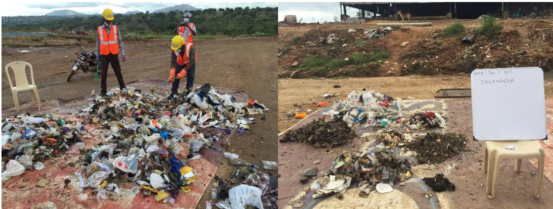
Figure 3-3: Quartering and Categorization of waste Sample
