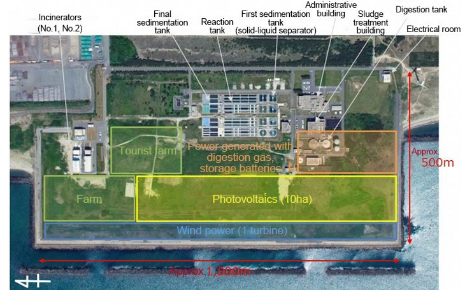
Layout of renewable energy facilities at Akita Rinkai Processing Center (Source: Akita Prefecture)
