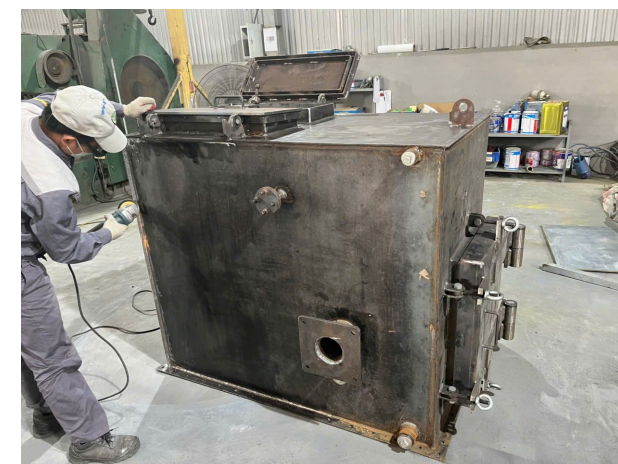
Prototype of small biomass boiler
