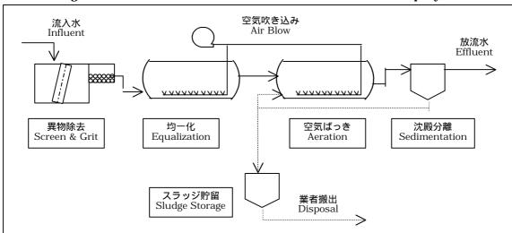
Figure 2-4-8 Planned Wastewater Treatment Plant of Company M
