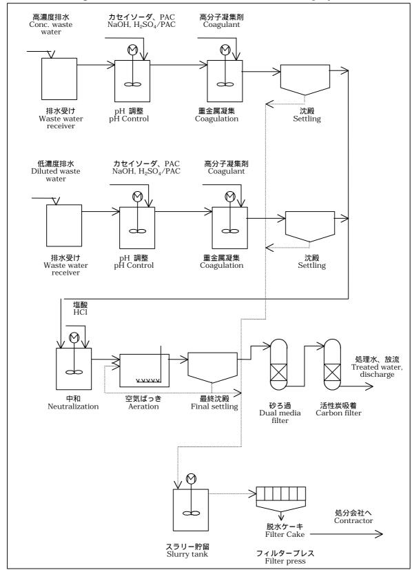
Figure 2-2-6 Flow of the Wastewater Treatment of Company B
