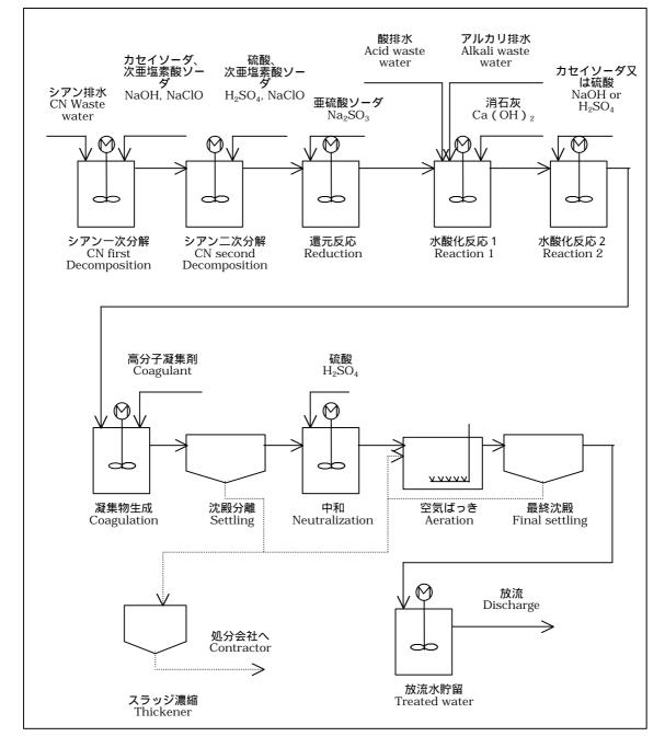
Figure 2-2-13 Flow of the Wastewater Treatment of Company D
