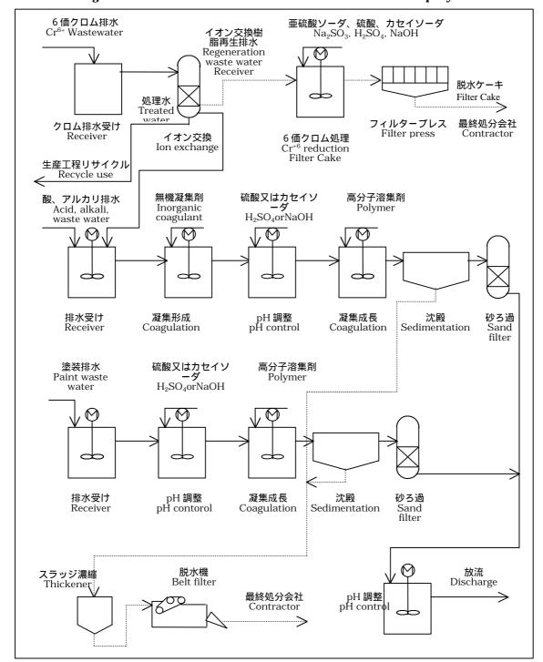
Figure 2-4-4 Flow of the Wastewater Treatment of Company K
