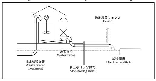
Figure 2-4-5 Facilities for Underground Water Monitoring
