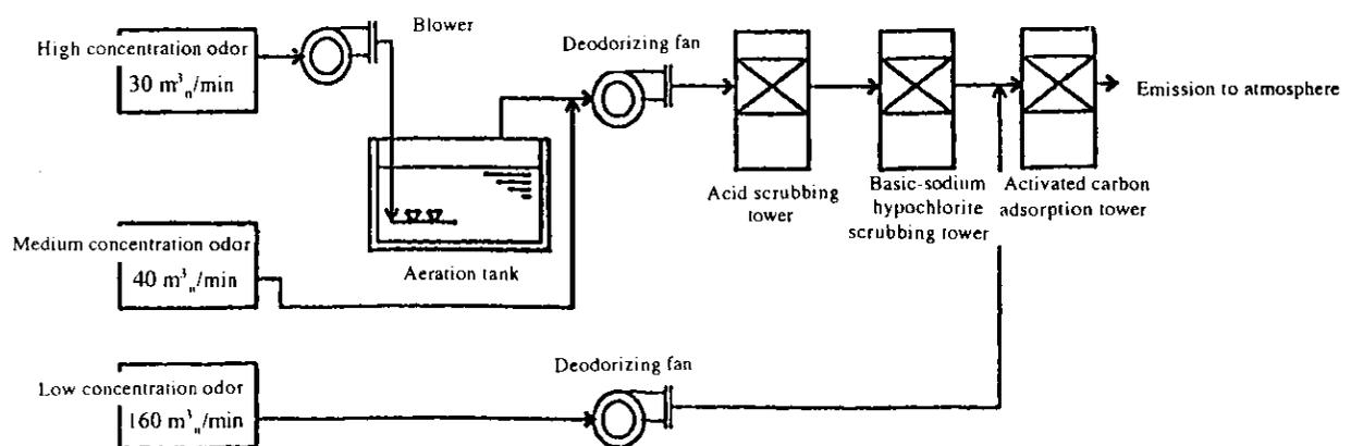
Fig.7.13.1 Examples of Deodorization Method at Night Soil Treatment Facility<sup>1)</sup>
