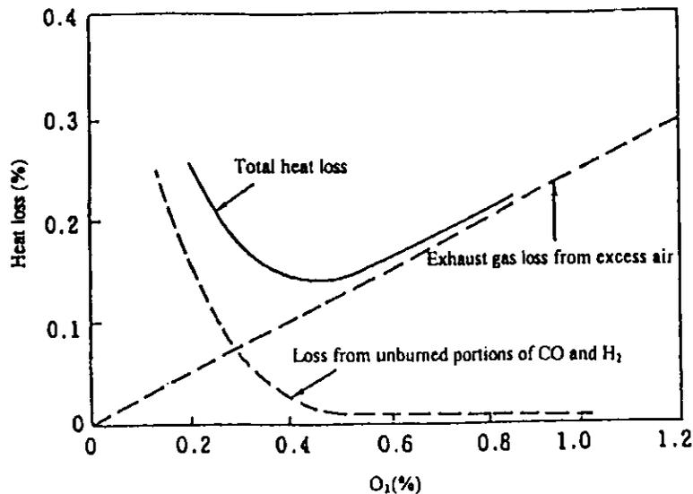
Fig. 7.4.1 Relationship between O<sub>2</sub> concentration and total heat loss
