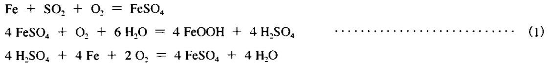
This structure is called auto-catalytic, the reaction repeatedly produces FeOOH and promotes corrosion.
