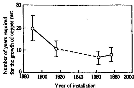
Fig.5.3.2 Number of years required for the growth of copper rust on copper surfaces installed each year in the eastern United States
