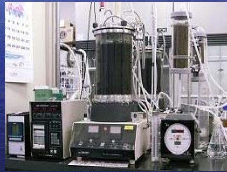
Seaweed biomass utilization (anaerobic digestion to produce methane gas)
