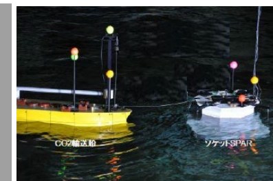
Aquarium test of offshore facility for injection
