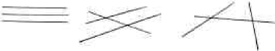
Count bundles as 1 structure; 1 or more parallel fibrils less than 1 fiber diameter separation.
