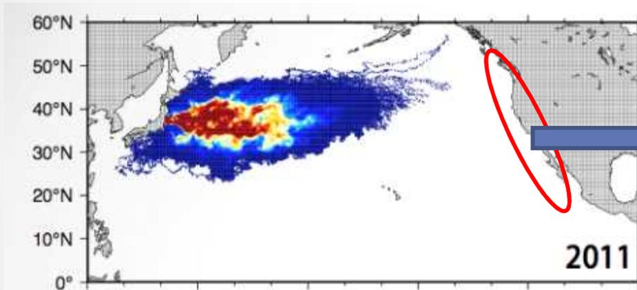
**Sub-model** based on the two rules associated with satellite winds at the nearest grid cell to reproduce the debris washing ashore and re-drift (nearshore processes).
