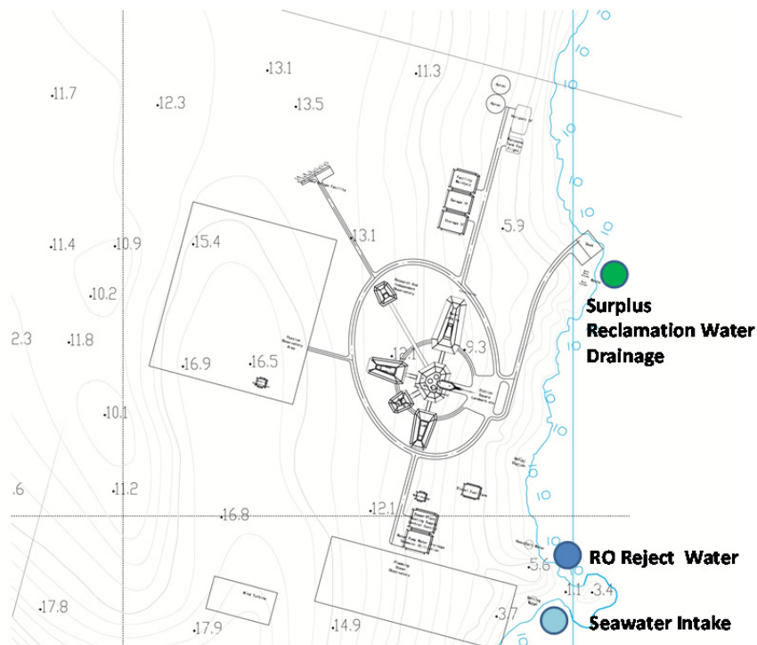
Figure 2-14 Intake and drainage locations
