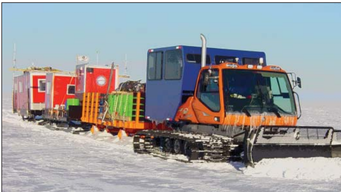
Figure 22. The tractor and sledge used to transport equipment and fuel to the drill site.
