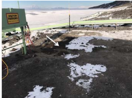
Hydrocarbon staining in parking area
