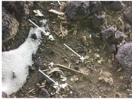
Visible ACM fragments under the Administration building
