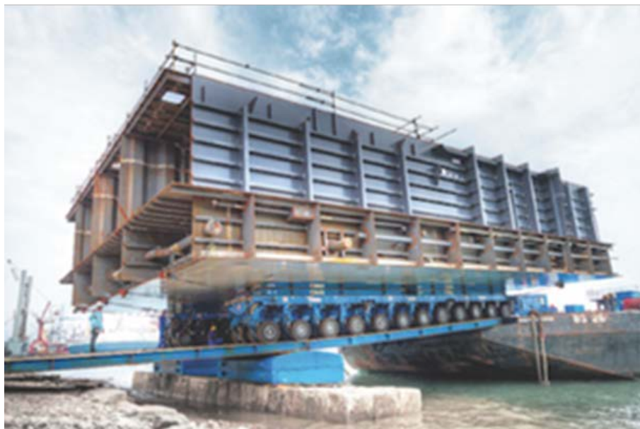
Figure 46: Example of SPMT crossing from ship to shore.
