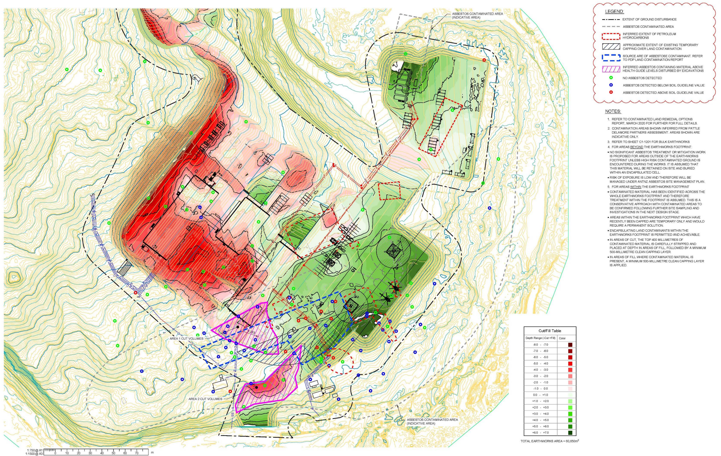
Figure 32: Plan showing the cut (red) and fill (green) profile with contamination areas both known and inferred superimposed (WSP, 2020).
