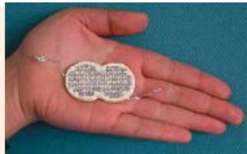
Ceramic thermo-electric module composed of 140 pairs of thermo-electric junctions Photo: courtesy of National Institute of Advanced Industrial Science and Technology (AIST)
