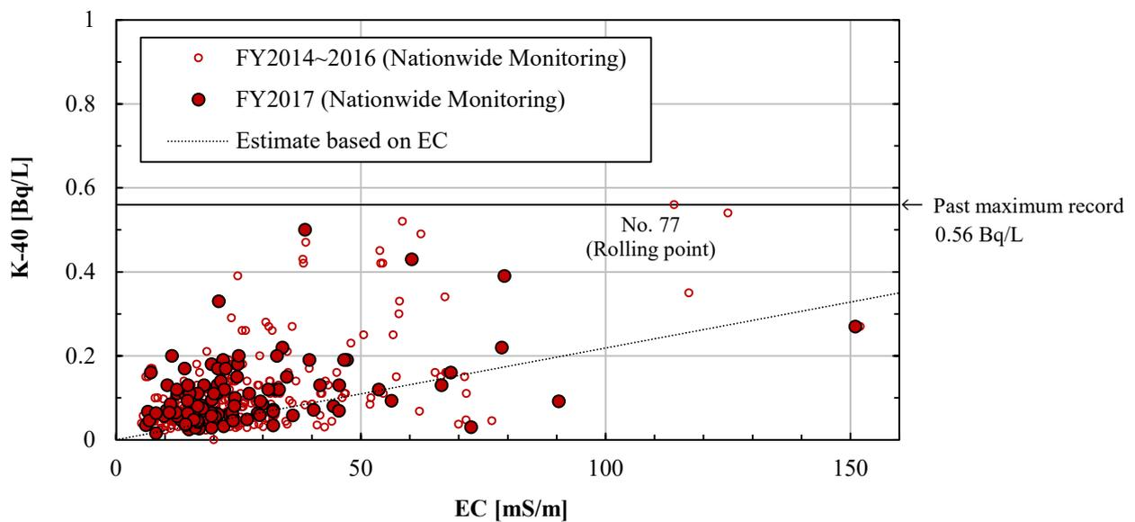
Figure 3.2-2 Correlation between the K-40 concentration and electrical conductivity (EC) in groundwater
