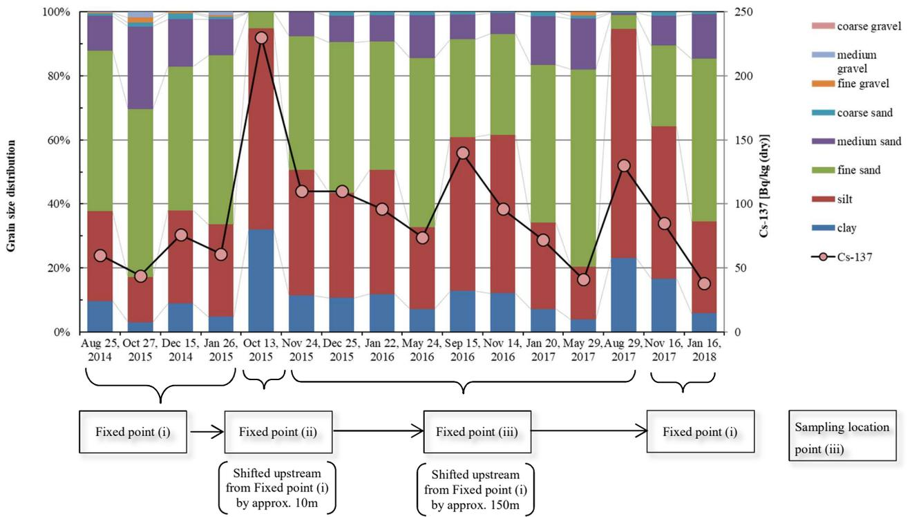
Figure 3.3-3 Changes in sediment grain size distribution and Cs-137 concentration [River No. 28]
