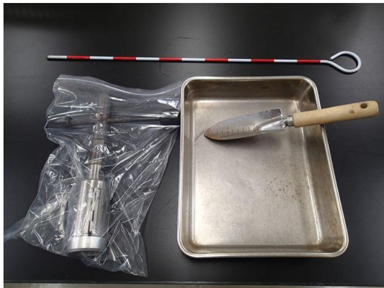
Figure 3. Soil sampler kit.
