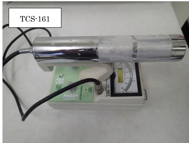
Figure 5. NaI (Tl) scintillation survey meter
