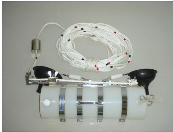
Figure 7. Van Dorn sampler
