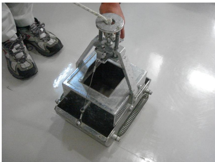
Figure 2. Ekman-Birge bottom sampler
