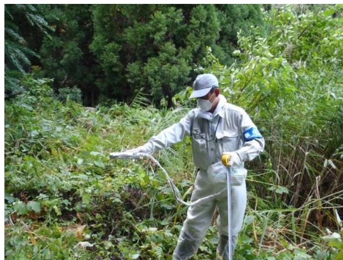
Figure 6. Measurement of ambient dose rates (example)
