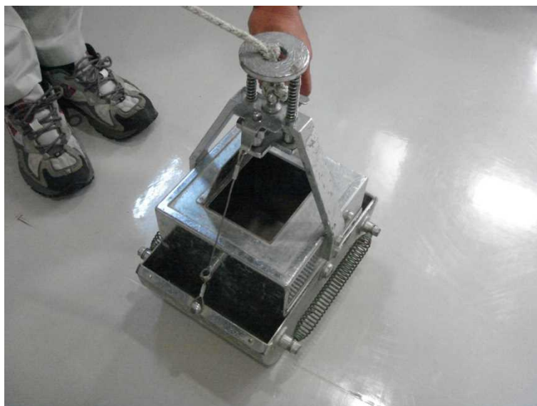
Figure 2. Ekman-Birge bottom sampler
