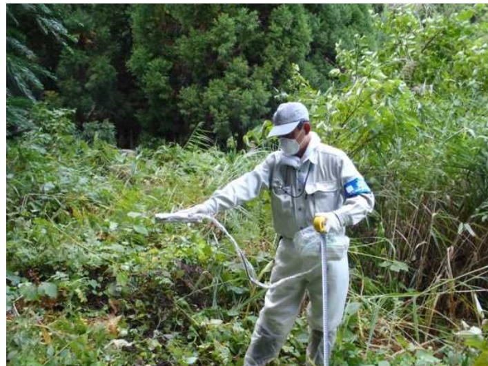
Figure 6. Measurement of ambient dose rates (example)
