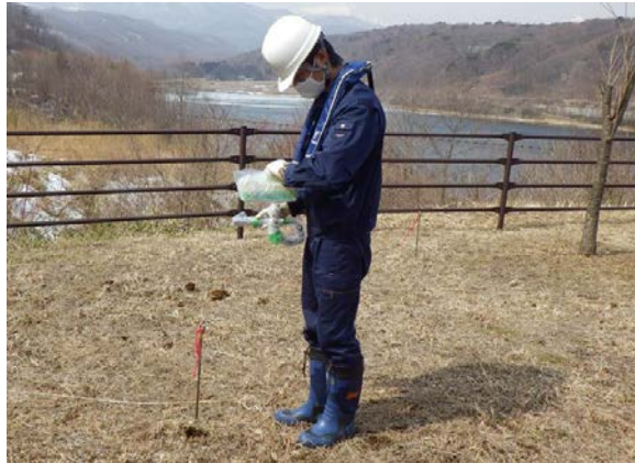
Figure 4 Measurement of Spatial Dose-rate (Example)
