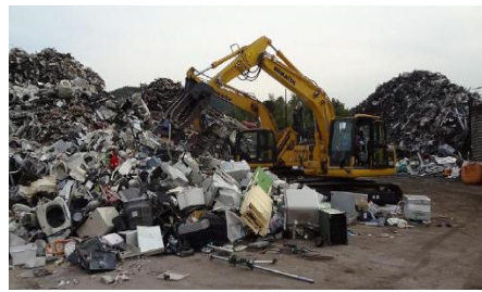
Yard suppliers destroy electric appliances without taking environmental measures, discharging hazardous substances such as Freon gases into environment.
