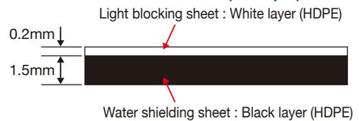
A water shielding sheet covers the floor and sloped surfaces of the controlled landfill site to prevent the pollution of underground water. Sheets with outstanding durability are being developed and used.
