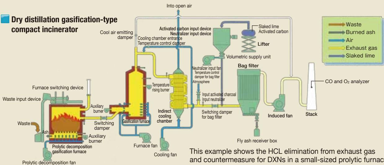
This example shows the HCL elimination from exhaust gas and countermeasure for DXNs in a small-sized polycyclic furnace.
