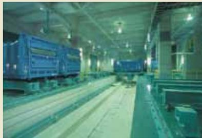
Garbage collected by small garbage trucks is dropped in a hopper, compressed in containers and reloaded onto larger trucks. In this transfer station, garbage collected by three 2-ton trucks can be compressed in one container. The container is then transported to a disposal site or incineration plant on a large container truck.
