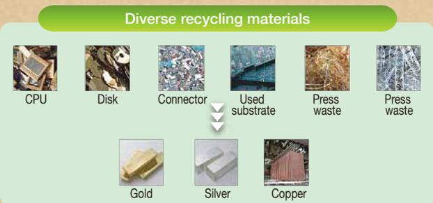
In collaboration with the nonferrous refining industry, heat and chemical treatments recover useful metals of high purity. Research is also conducted to develop technology to recover and use rare metal in the future.
