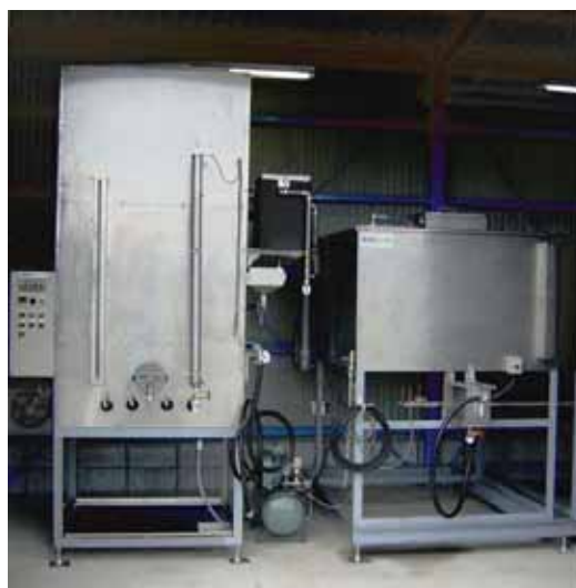
Figure 5.2-4 Photos of the Distillation Reclamation Facility for Liquid Refrigerant
