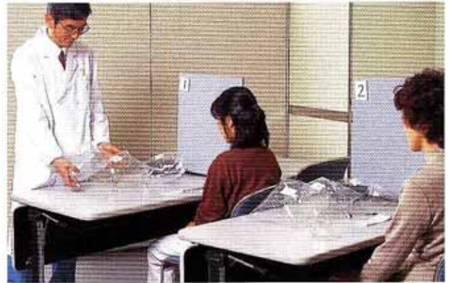
Panel members are to identify the bag with odor among 3 bags in a composed environment without odor where they can concentrate on the test.
