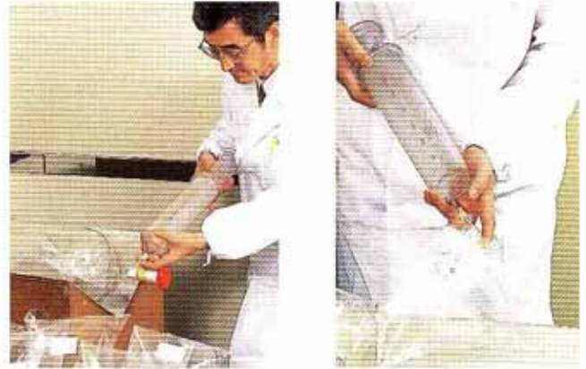
When panel members detect intensive odors, their olfaction weakens (olfactory fatigue). Therefore, the test is started with a moderately diluted concentration.
