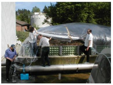
Fig. 1 Sampling at an active area source - biofilter
