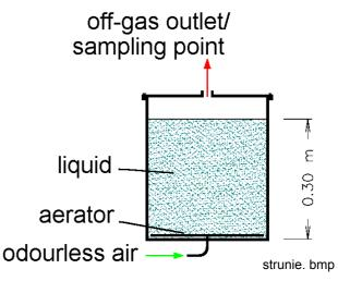
Fig. 5 sketch of the OEC test reactor
