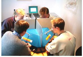
Fig. 4 Example of a four-sniffing-place yes/no olfactometer (in total 4 sniffing ports)
