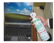
Air dusters, which emit a jet of high pressure gas, are used widely in maintenance of office appliances (computers, office automation equipment etc.) as well as precision equipment in factories and laboratories (electronic and optical equipment etc.), ATMs in banks and convenience stores, and automatic ticket gates etc. in stations, with the purpose of removing dust and static electricity and cooling the object. The demand for air dusters has grown strongly in parallel with the popularization
