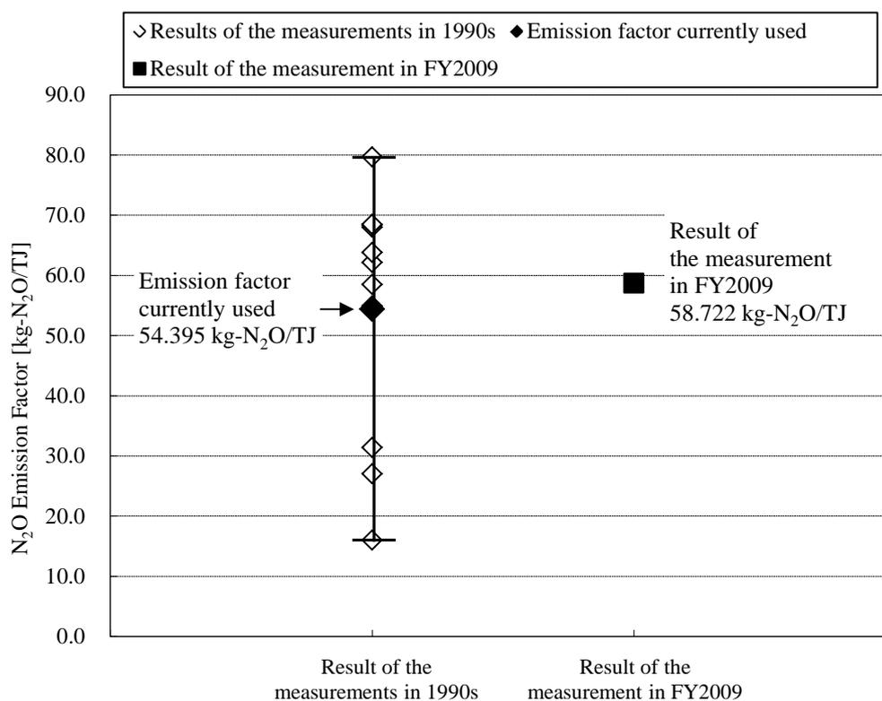
Figure 3-6 Comparison of the 1990s and FY2009 measurement results
