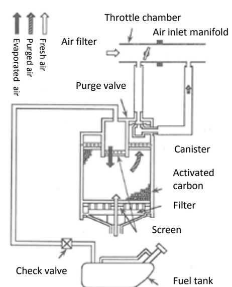
Source: Technology of engine in vehicle for environment, Society of Automotive Engineers of Japan
