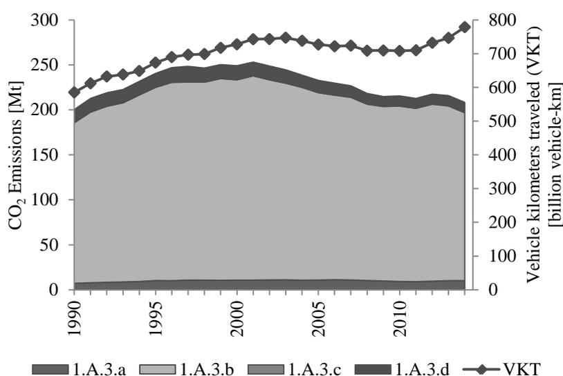
Figure 3-8 The trends of CO<sub>2</sub> emissions from Transport (Mobile Combustion) (1.A.3.) and related indicator
