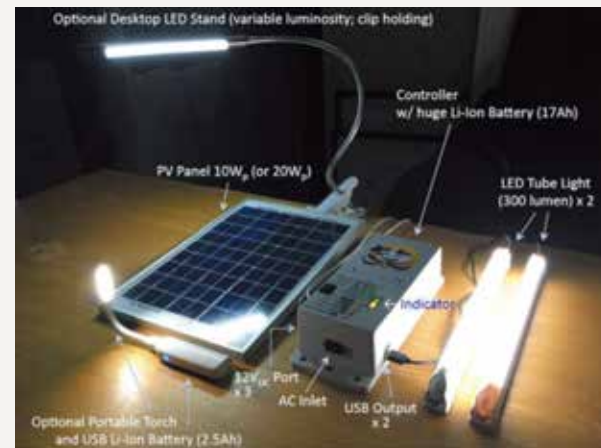
Figure 20 Example of project under “Subsidy program for innovation of low carbon technologies for developing countries”: Micro-scale photovoltaic technology for non-electrified regions by PEAR Carbon Offset Initiative, Ltd. (Source: Ministry of the Environment, Japan)
